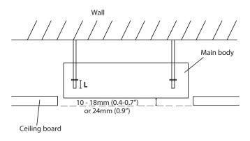
**NOTE**: The bottom of the unit should be 10-25mm(0.4-0.98")higher than the ceiling board. Generally, L (indicated in the following figure) should be half the length of the suspension bolt or long enough to prevent the nuts from coming off.
