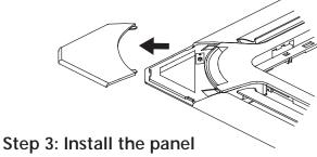
Align the front panel to the main body, taking into account the position of the piping and drain sides. Hang the four latches of the decorative panel to the hooks of the indoor unit. Tighten the panel hook screws evenly at the four corners.
