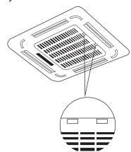
Step 2: Remove the installation covers at the four corners by sliding them outwards.
