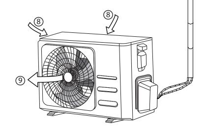
(B) 1 (7)1 Air outlet 2 Air inlet 3 Front grille 4 Display panel S Remote controller 6 Drain pipe Connecting pipe Air inlet 8 Air outlet
