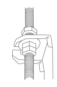
**NOTE**: The bottom of the unit should be 10-18mm(0.4-0.7")(Super-Slim models) or 24mm (0.9")(Compact models) higher than the ceiling board. Generally, L (indicated in the following figure) should be half the length of the suspension bolt or long enough to prevent the nuts from coming off.
