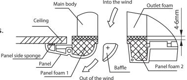
**NOTE**: If the height of the indoor unit needs to be adjusted, you can do so through the openings at the panel's four corners. Make sure that the internal wiring and drainpipe are not affected by this adjustment.
